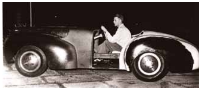
A nineteen year old Seward Allen being "fitted" in car during construction in 1939-1940. Note the floor pan well below the chassis rail.
